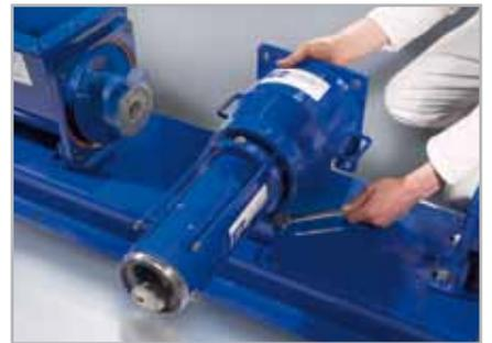
**6. Unscrew the rotor from the stator**
