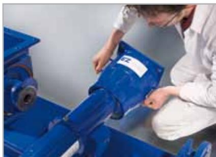
**8. Remove the stator**
